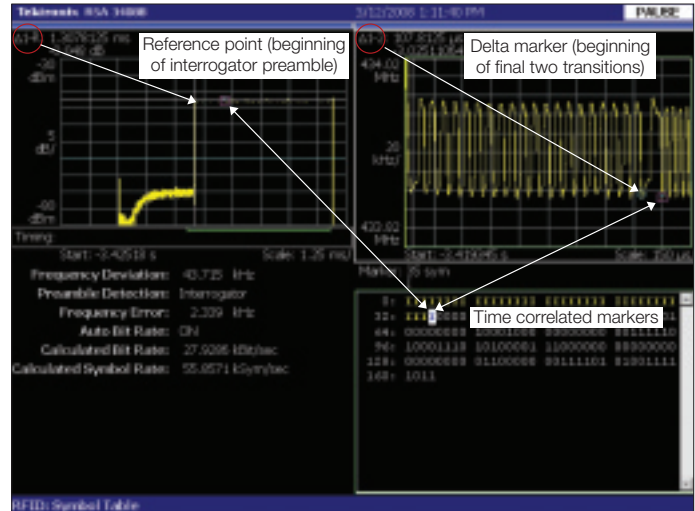
Figure 20. Verifying preamble of an ISO18000-7 Interrogator ('I') signal using time-correlated markers (special thanks to Savi Technology).
